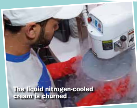
The cream is cooled with liquid nitrogen applied from the outside
